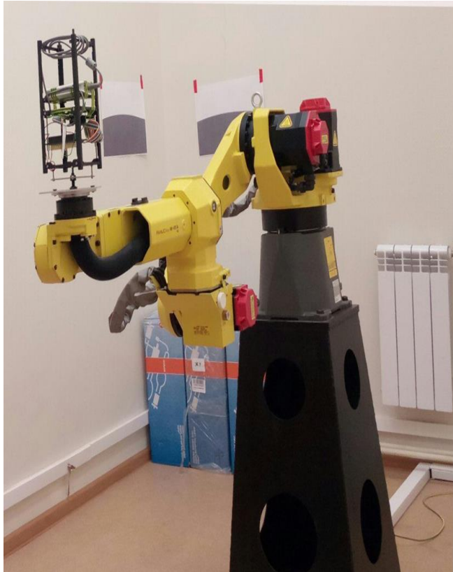
The nanosatellite, mounted on manipulator
