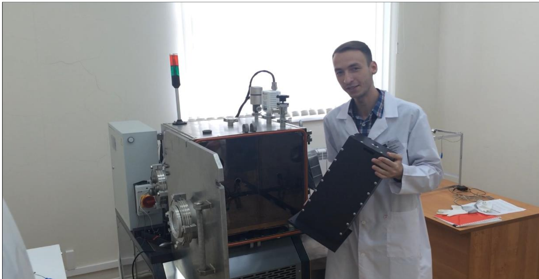
The housing for testing the thermal Cycling
